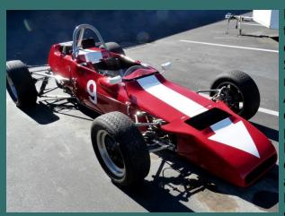
Professionally built and maintained throughout its life. Comprehensively overhauled in the spring of 2013. Stripped to bare chassis, crack checked, repaired and powder-coated. New Aluminum floor. It has a fresh Ivey engine, new fuel cell, new seat, fresh paint, widened body at shoulders, new Penske shocks and new springs, rod ends, suspension bolts, donuts, oil tank and lines, and much more detail work. Fully set up, corner-weighed, bumpsteered etc. Four race weekends since
