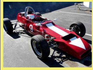
Professionally built and maintained throughout its life. Comprehensively overhauled in the spring of 2013. Stripped to bare chassis, crack checked, repaired and powder-coated. New Aluminum floor. It has a fresh Ivey engine, new fuel cell, new seat, fresh paint, widened body at shoulders, new Penske shocks and new springs, rod ends, suspension bolts, donuts, oil tank and lines, and much more detail work. Fully set up, corner-weighed, bumpsteered etc. Four race weekends since
