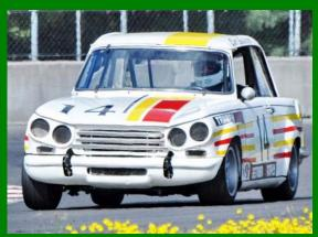
British Leland Factory car prepared by Kastner for the 1971 series. A fresh TR6 2.5 engine with 3 Webers measuring 211 HP at the rear wheels and a Housen 5-speed. Upgraded suspension & lots of spares. Including race prepared 2.0 GT6 engine and TR6 transmission with Dolom CR gears plus a second set of Panasport \$45,000. Sharon Gilbert: 209-894-3949 email: bsgil99@hughes.net
