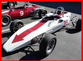
Vintage Formula Ford chassis #4. We have had the car since 2011 and raced it eight weekends. It has an Ivey engine that was fresh when we got the car. The gearbox is a Webster/Hewland. The suspension has just been completely rebuilt after a 3 car tangle in 2014. The bodywork has just been stripped and repainted. It has a new nose cone and a spare. It has just been fully corner-weighed bump-steered and aligned. This car is fully race prepped and ready to go. It is an
