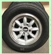
Five, thirteen inch diameter wheels. Lug pattern is 4 X 4 1/4. Width is 7". The wheels, stamped "for racing only" are in very good to excellent condition. These wheels should fit many, if not all, of the cars that utilize a Spitfire/GT6 hub. Four of the wheels have Toyo R888 205/60/13 tires that have been used for a couple of races. All five wheels with tires \$600 or \$500 without tires. Contact Mike at 831-345-3955
