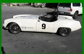
Originally Built by Don Kopiski: Items include: New bodywork; New MGB 1800 engine Built by John Davis at Epifani Restorations Rebuilt MGC close ratio gearbox; new interior; new wheels; new brakes; new Tilton pedal box; new exhaust built by Tom Smith; new seat; newbelts; new alternator & distributor, new Weber carb. Professionally bumpsteered and aligned. One test day at Sears point since
