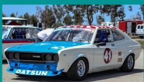
1974 Datsun 710 B-Sedan, \$25,000. Race prepped I20b engine, approx 200hp. Close-ratio 5 speed. LSD. 8point cage. Disc front/drum rear brakes. Coilover front, panhard/leaf/coil rear. Fresh tires, brakes, oils. Ready for the 2019 B-Sedan/Trans-Am 2.5 season. Contact Troy at:
