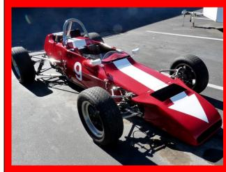
Professionally built and maintained throughout its life. Comprehensively overhauled in the spring of 2013. Stripped to bare chassis, crack checked, repaired and powder-coated New Aluminum floor. It has a fresh I engine, new fuel cell, new seat, fres paint, widened body at shoulders, ne Penske shocks and new springs, rod ends, suspension bolts, donuts, oil ta and lines, and much more detail worl Fully set up, corner-weighed, bumpsteered etc. Four race weekends sin
