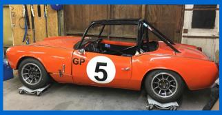
\$7000 OBO. Log books back to early 70's. All Steel Body. 8 Gal ATL cell is less than 5 years old. 10 pound fire sys. with 3 nozzles. GT6 brakes/suspension on all 4 corners. Muller race axles in rear. Koni red shocks all corners. Alloy bell housing. Have build sheet on 1147cc engine in car. Car is a blast to drive, fast and
