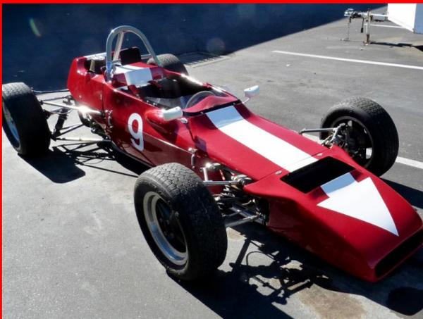
Professionally built and maintained throughout its life. Comprehensively overhauled in the spring of 2013. Stripped to bare chassis, crack checked, repaired and powder-coated. New Aluminum floor. It has a fresh I engine, new fuel cell, new seat, fresh paint, widened body at shoulders, new Penske shocks and new springs, rod ends, suspension bolts, donuts, oil tank and lines, and much more detail work. Fully set up, corner-weighted, bump-steered etc. Four race weekends since
