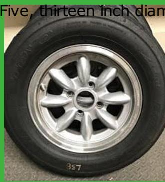
Five, thirteen inch diameter wheels. Lug pattern is 4 X 4 1/4. Width is 7". The wheels, stamped "for racing only" are in very good to excellent condition. These wheels should fit many, if not all, of the cars that utilize a Spitfire/GT6 hub. Four of the wheels have Toyo R888 205/60/13 tires that have been used for a couple of races. All five wheels with tires \$600 or \$500 without tires. Contact Mike at 831-345-3955
